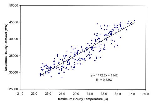
Fig. 5 Peak electricity demand in the Cal ISO area as a function of maximum hourly temperature: 2004–2005
