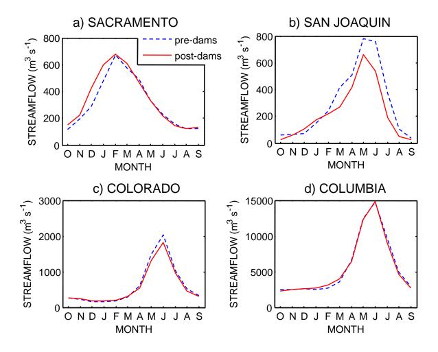
Figure 2. Streamflow climatologies of naturalized flow for two periods: pre and post construction of major dams in the rivers.
