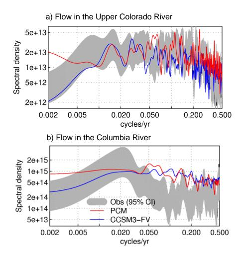
Figure 8. Power spectra of the streamflow at a) the Upper Colorado River at Lees Ferry and b) the Columbia River at the Dalles from the PCM and CCSM3-FV control runs compared to tree-ring reconstructions.
