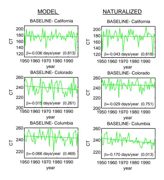
Figure 5. Time-series of the center timing (CT) of modeled (left panel) and naturalized streamflow (right panel) from 1950 to 1999. The values of the slope ( $\beta$ ) are shown, as well as the significance of the trend (in parenthesis). The values of CT are given in days from October 1<sup>st</sup>. The meteorological data used to force VIC is from Maurer et al. (2002).
