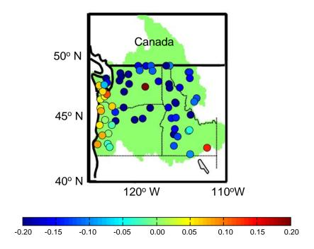
Figure 6. Trends in CT (days/year) from streamflow observations from 1950 to 1999 in the Columbia River Basin (CRB). The streamflow observations were obtained from the Hydro-climatic Data Network (HCDN) and updated from measurements from the United States Geological Survey. The CRB area is shown in green.
